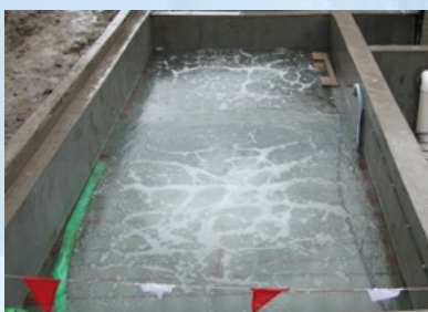
Figure 6 - "Ventus" aerator in operation
